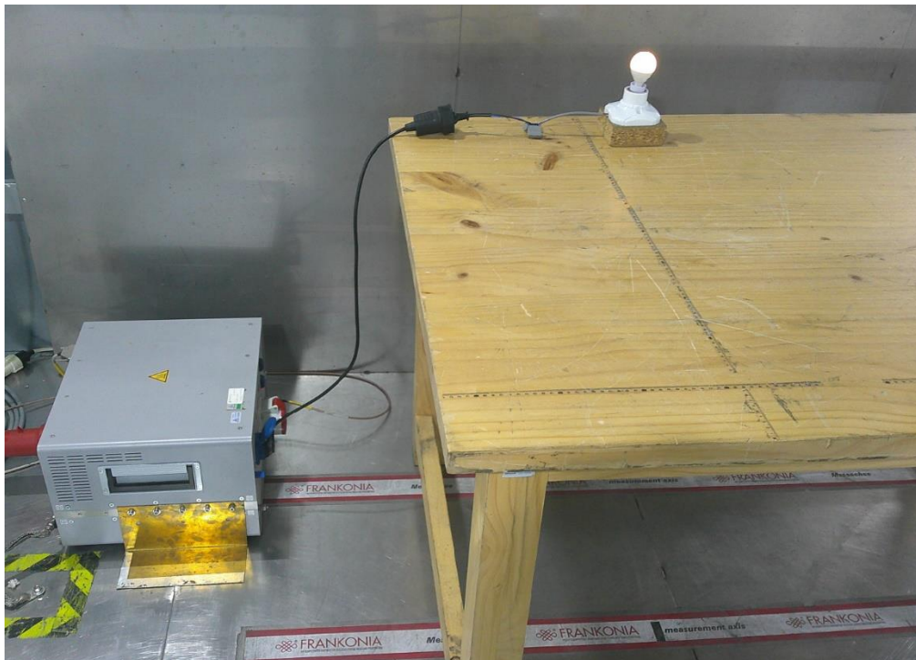
Photograph 2: Set-up photo for Conducted Emission
