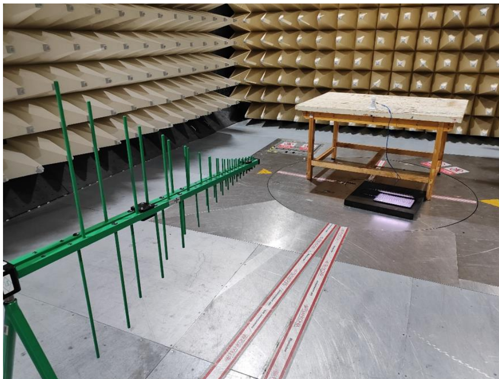
Photograph 3: Set-up photo for Radiated Emission, 30MHz - 1GHz
