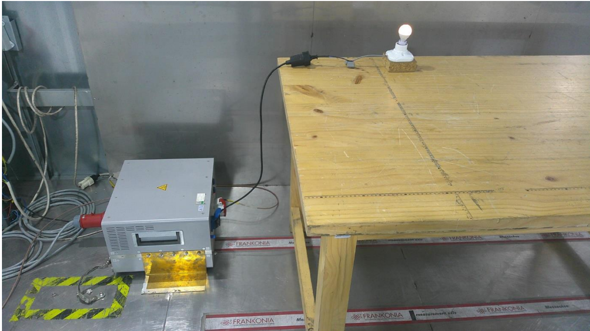
Photograph 2: Set-up for measurement of radiated emission
