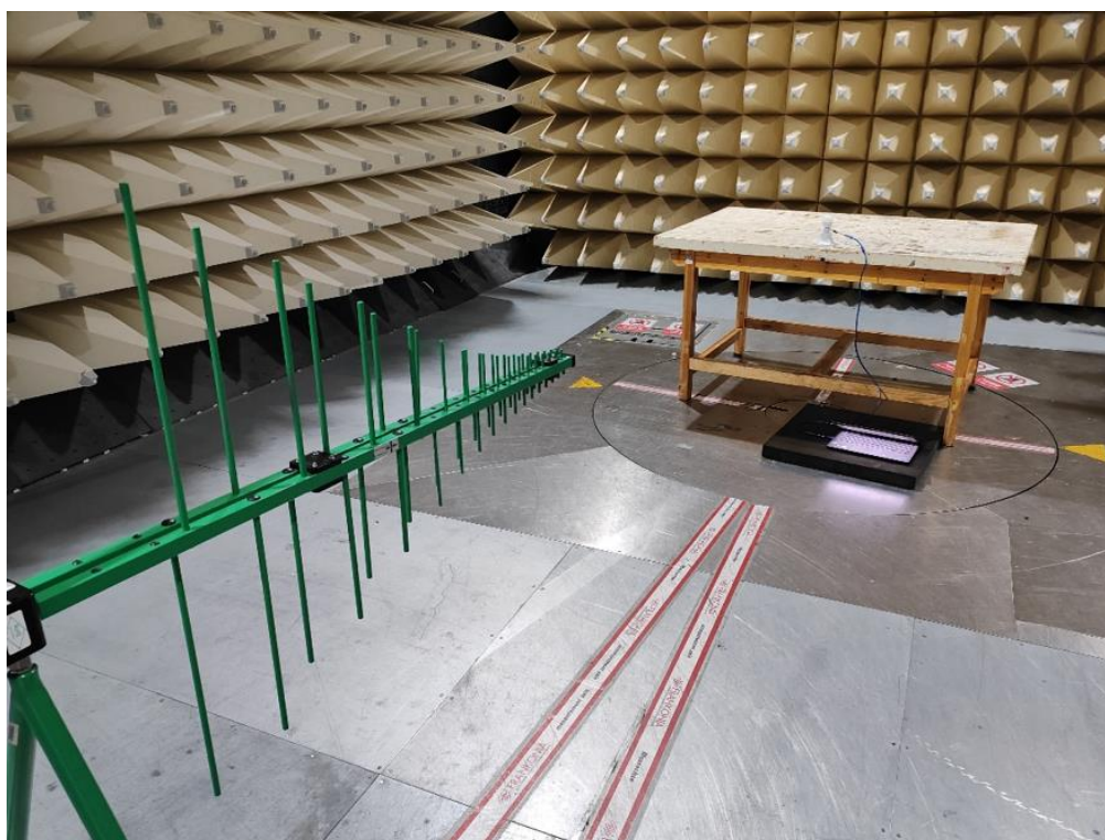
Photograph 3: Set-up photo for Radiated Emission, 30MHz - 1GHz
