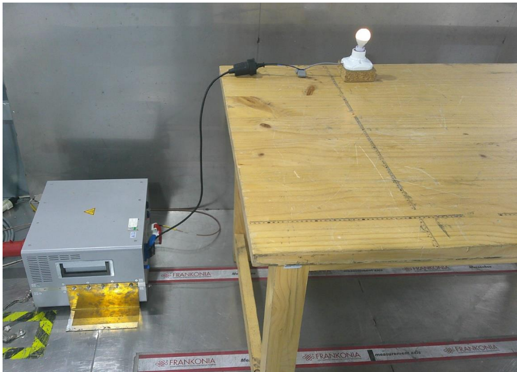
Photograph 2: Set-up photo for Conducted Emission
