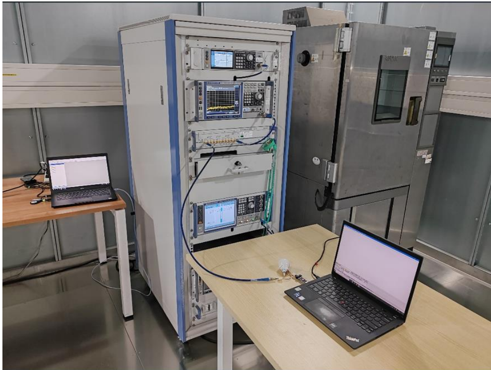
Photograph 1: Set-up photo for RF Conducted Test
