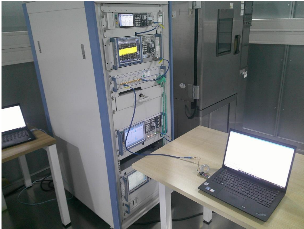
Photograph 1: Set-up photo for RF Conducted Test
