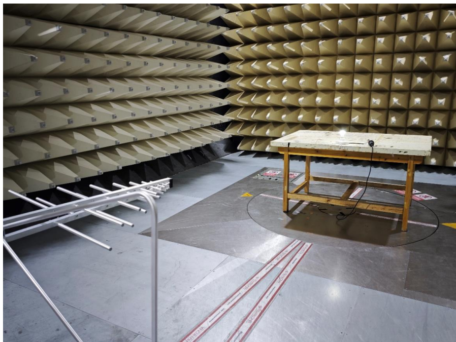
Photograph 2: Set-up for measurement of radiated emission
