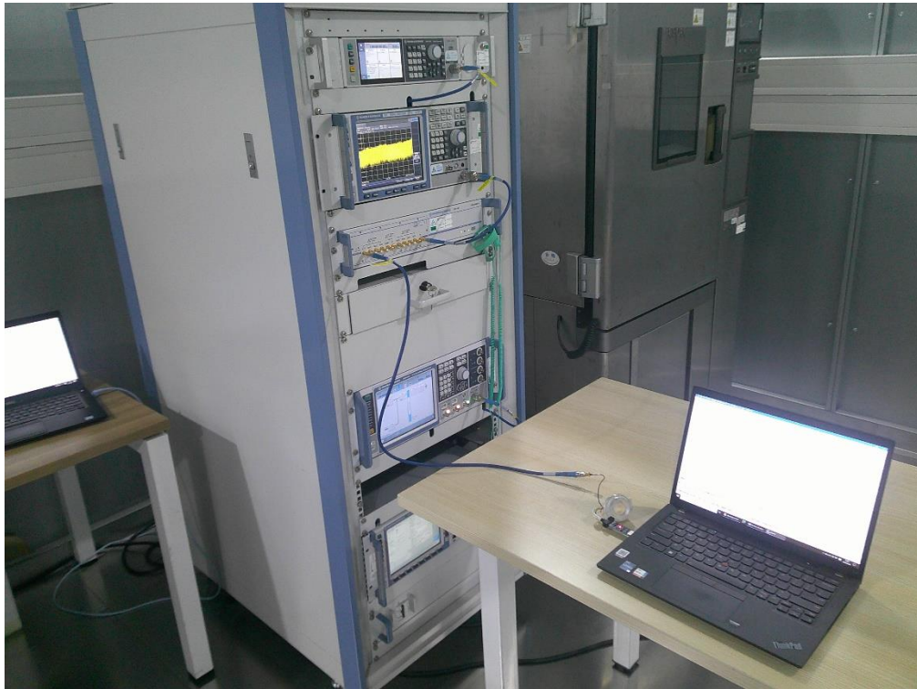
Photograph 1: Set-up photo for RF Conducted Test
