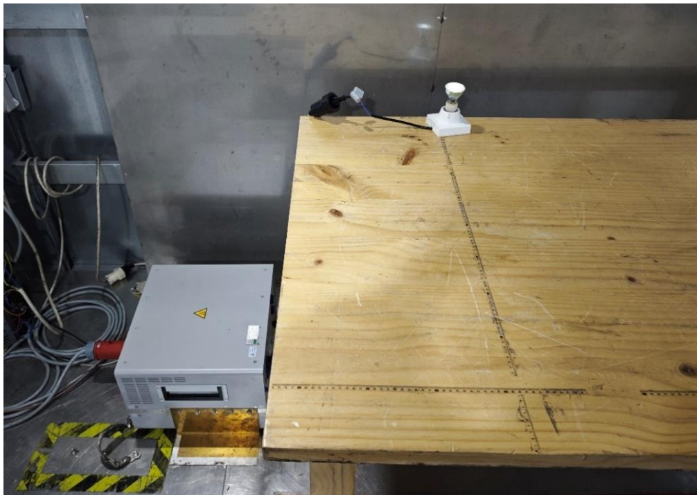
Photograph 2: Set-up photo for Conducted Emission
