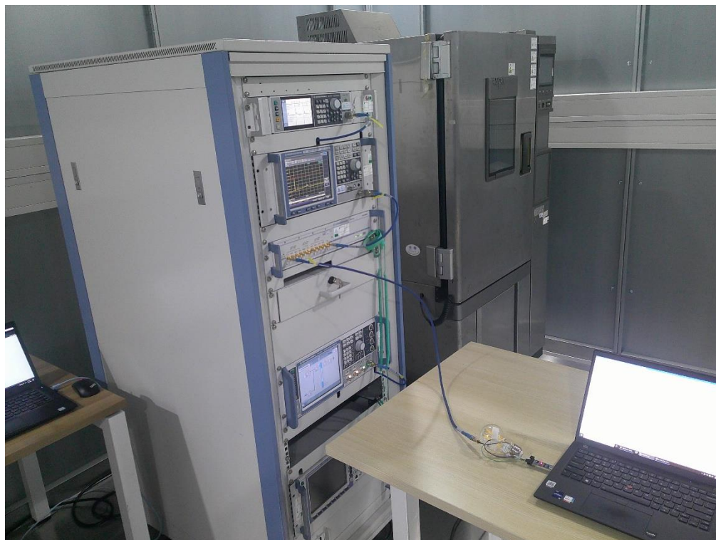
Photograph 1: Set-up photo for RF Conducted Test
