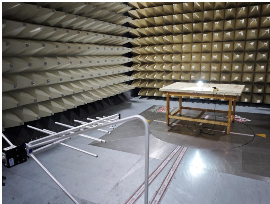
Photograph 2: Set-up for measurement of radiated emission
