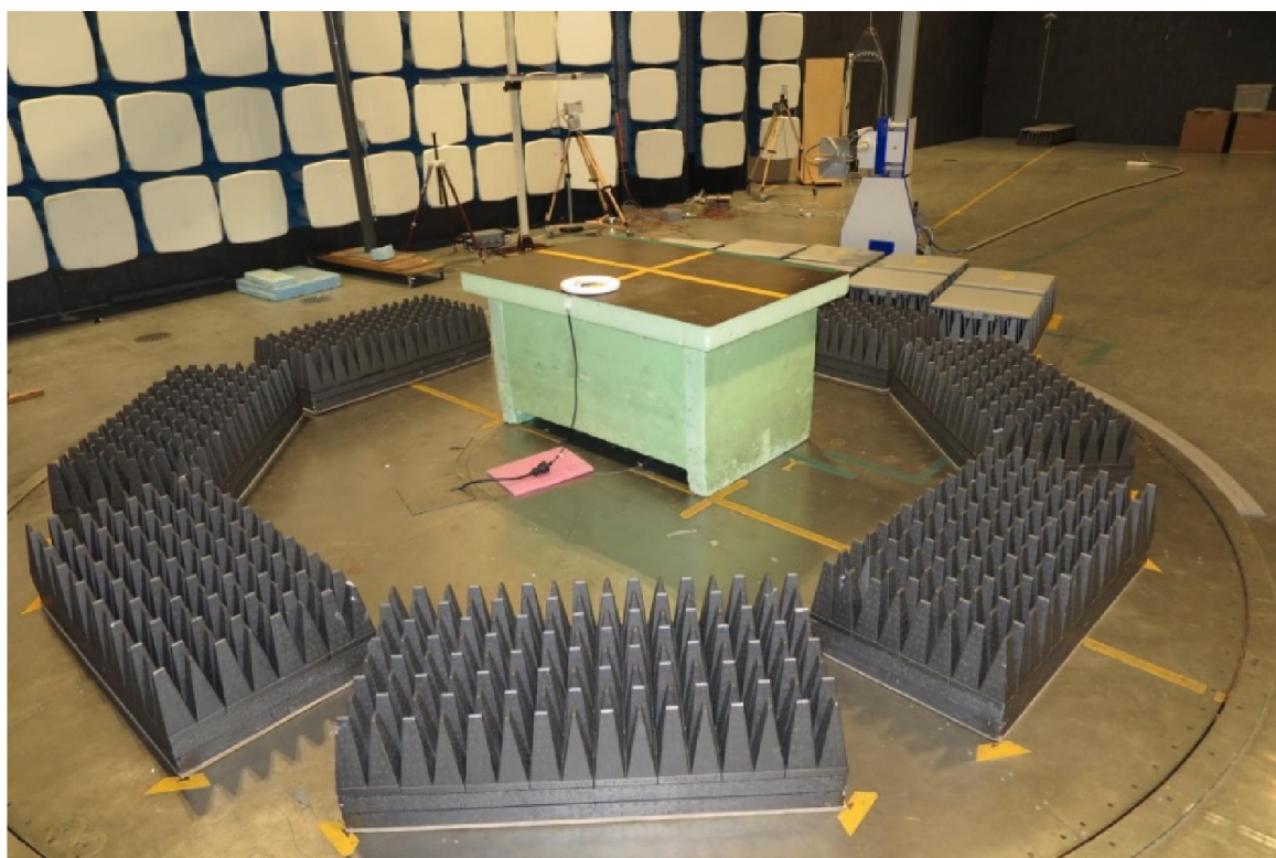
Test set up radiated emission 1 – 13 GHz
