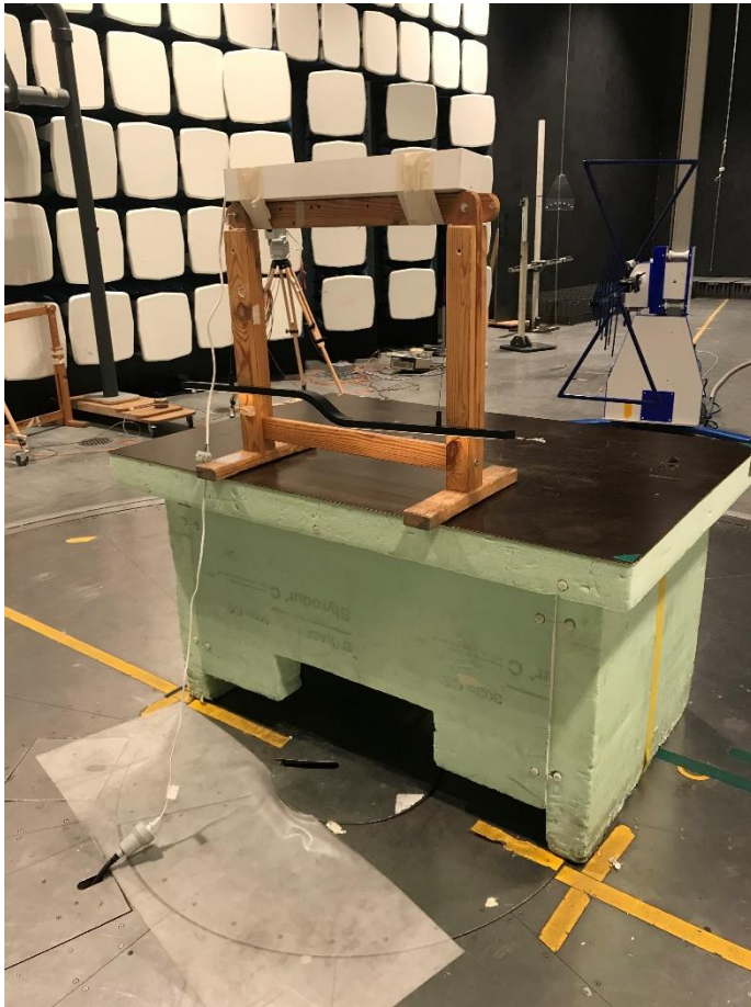
Test set up radiated emission 30 MHz – 1 GHz
