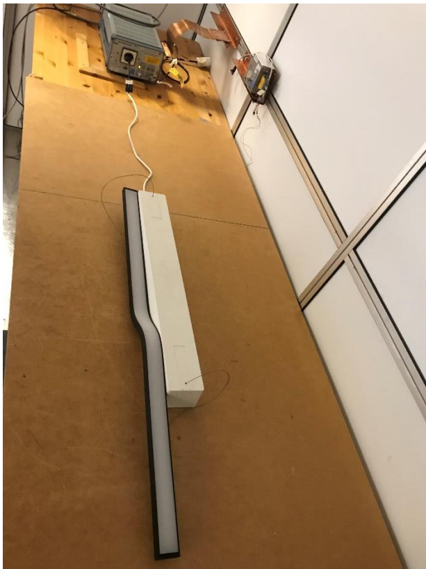
Test setup for conducted emission 150 kHz – 30 MHz
