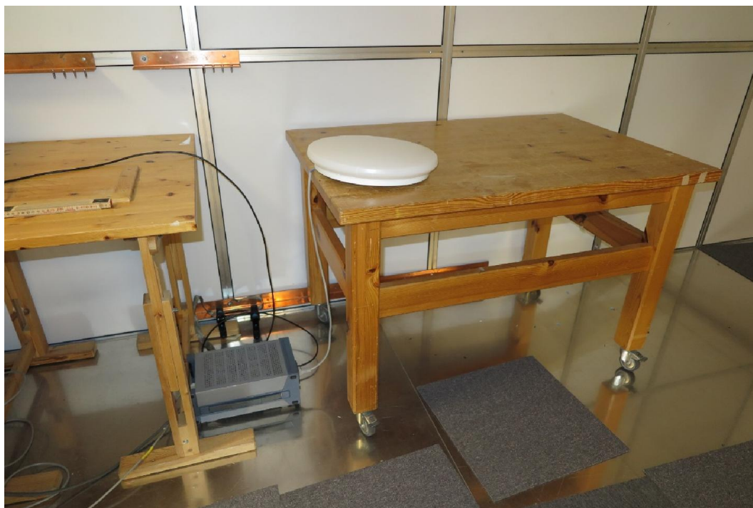
Test setup for conducted emission 150 kHz – 30 MHz
