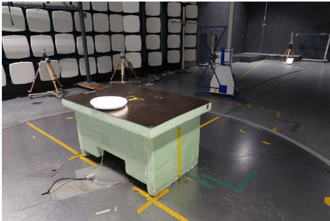
Test set up radiated emission 30 MHz – 1 GHz
