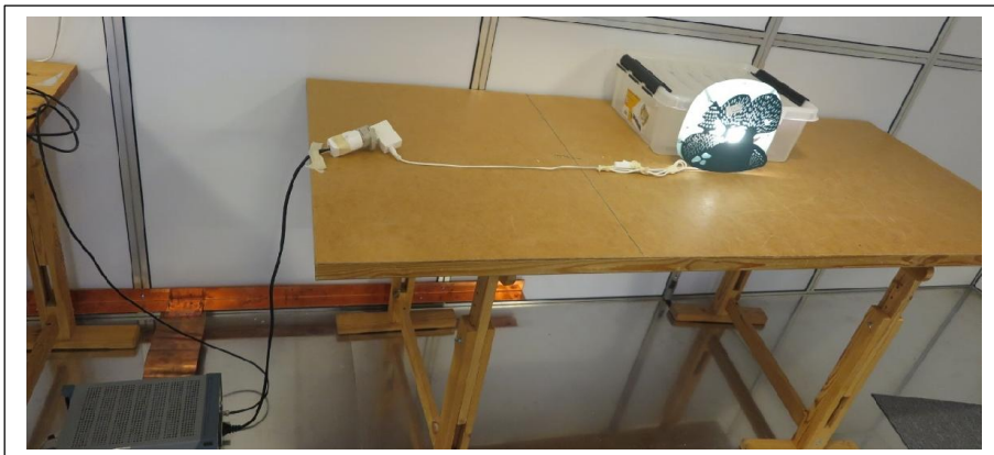
Test setup for conducted emission 150 kHz – 30 MHz
