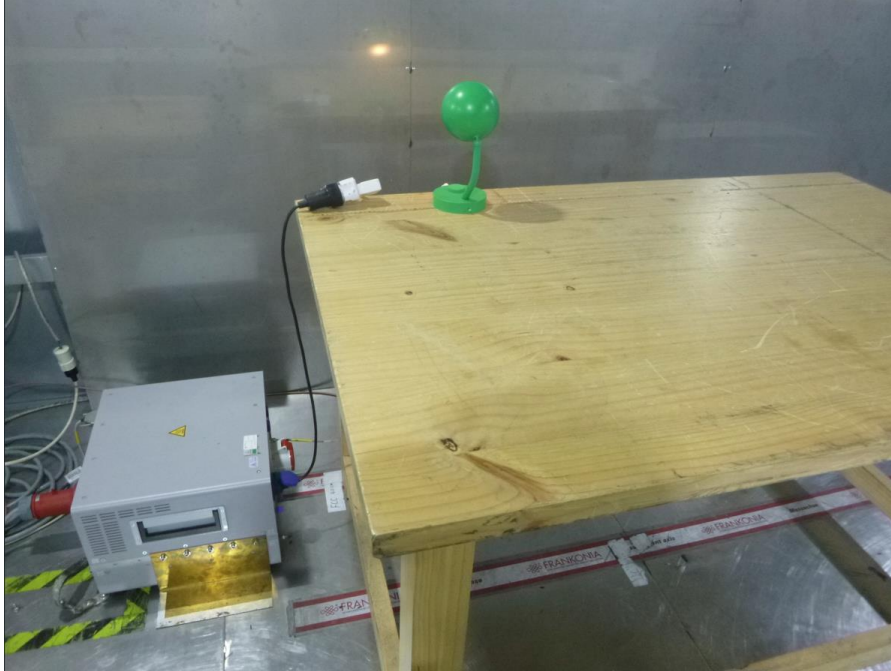
Photograph 2: Set-up for measurement of radiated emission
