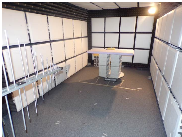
Test setup (9kHz-1GHz) for pre-scan measurement
