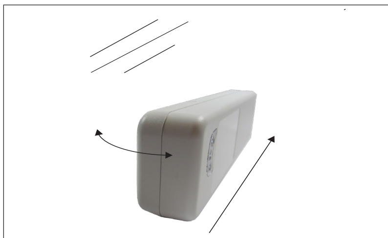
Figure 6 – Removing PocketPass from windshield
