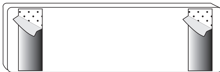
Figure 2 Peel backing from mounting strips to expose adhesive
