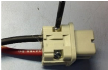
Figure 15 Thread Wires Through Assembly
