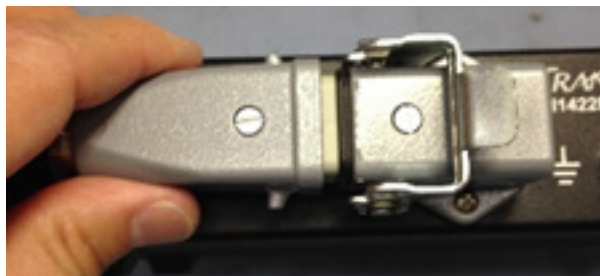
Figure 23 Remove Plug from Receptacle
