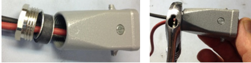
Figure 18 Reassemble Cable Gland Assembly
