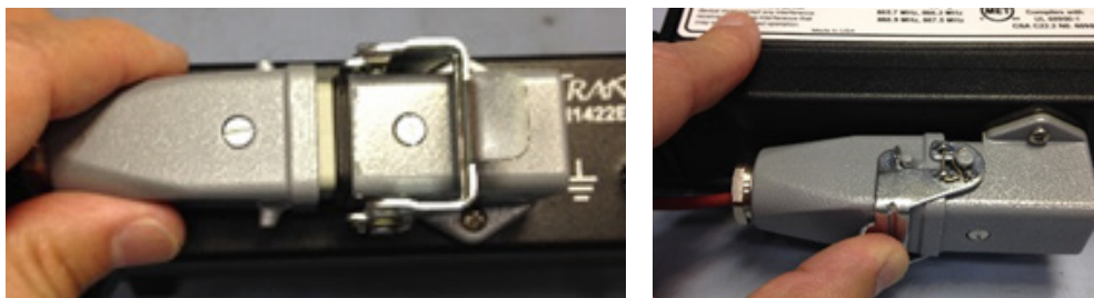
Figure 20 Reinstall Power Connector
