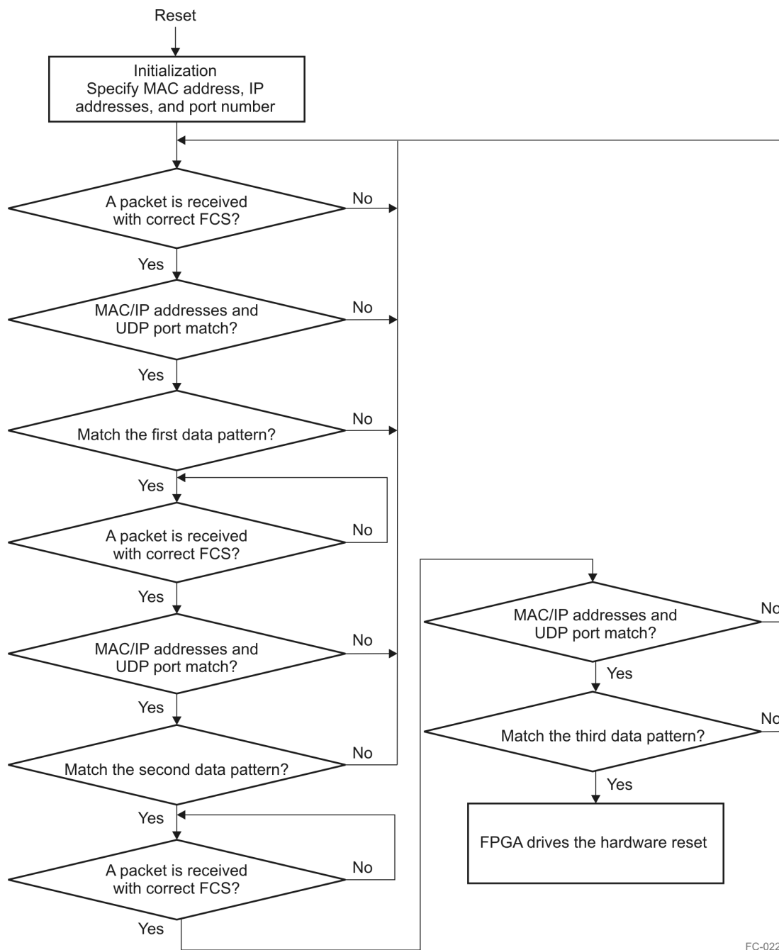
Figure 11-2 Remote Reset Control Operation Flow Chart
