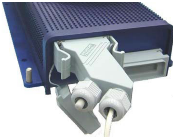
Figure 11–8 Check Tag Assembly Secured to MPRX Port
