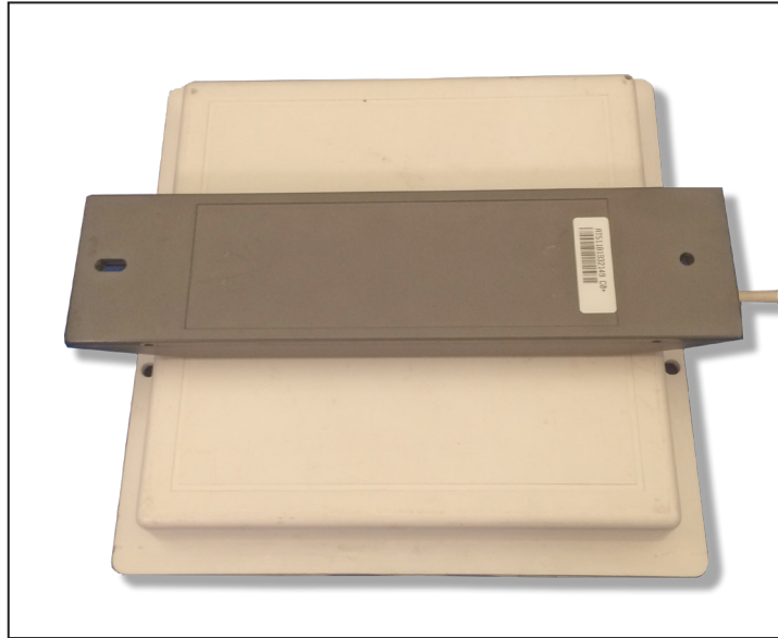
Figure 22 Tag and Antenna Orientation (horizontal polarization)
