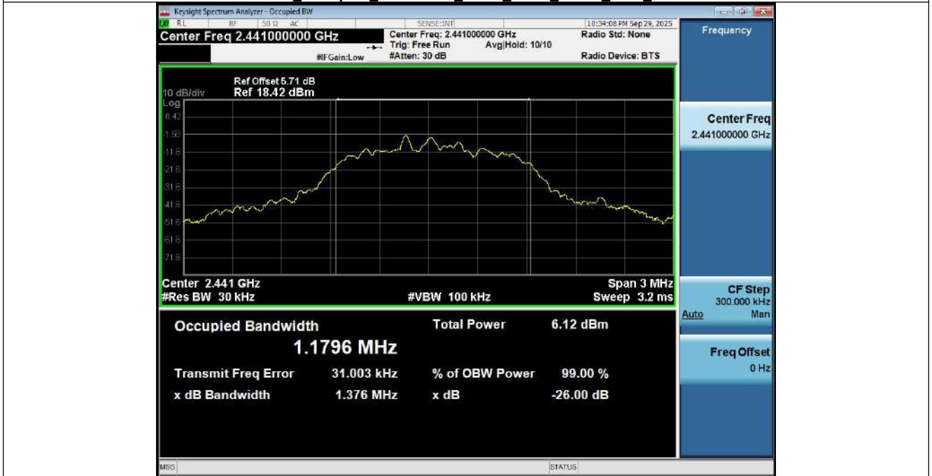
99% Occupied Bandwidth NVNT_ANT1_3-DH1_2441_00
