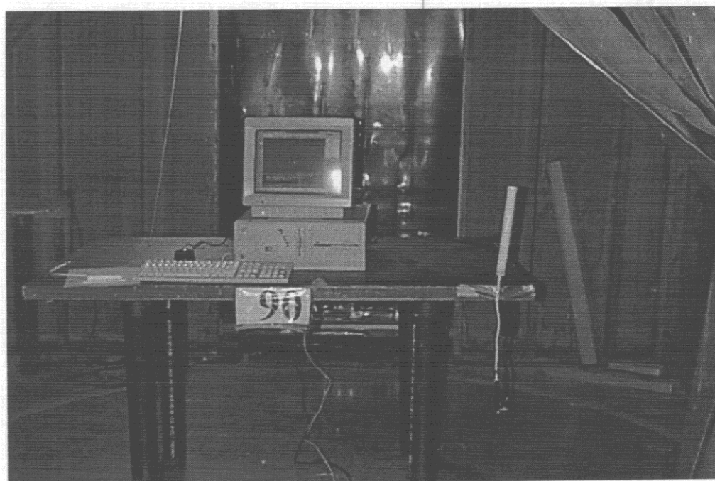
15.205 Restricted Band Test Setup Mobile Mark 9dBi Omnidirectional Antenna
