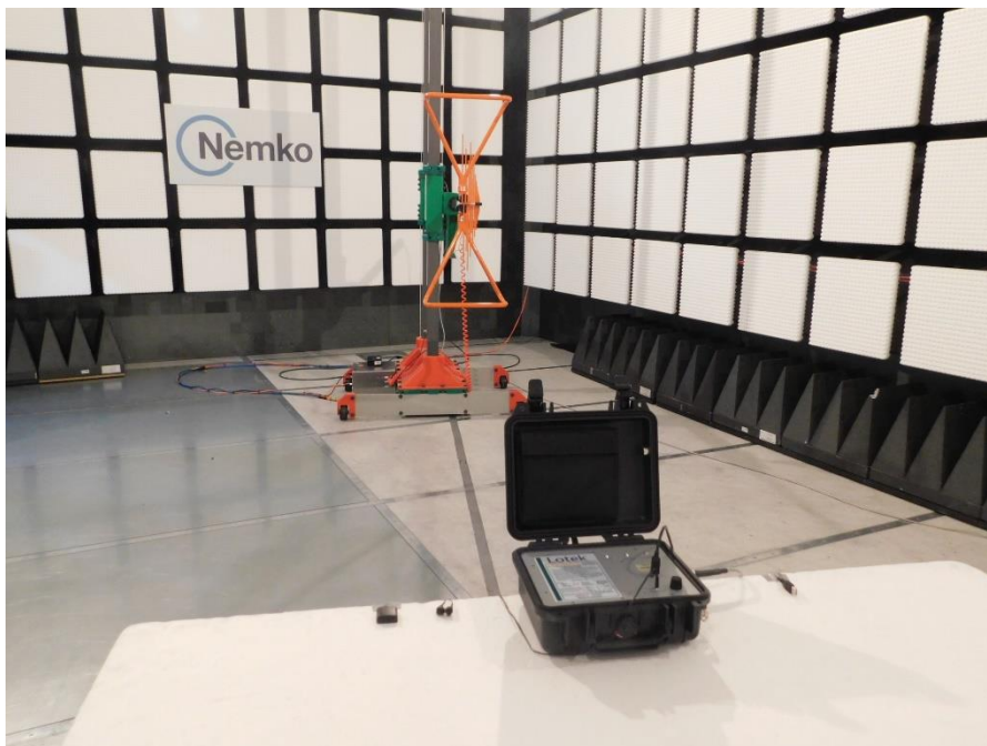
Figure 8.1-40: Radiated disturbance setup photo (SRX1200-D)
