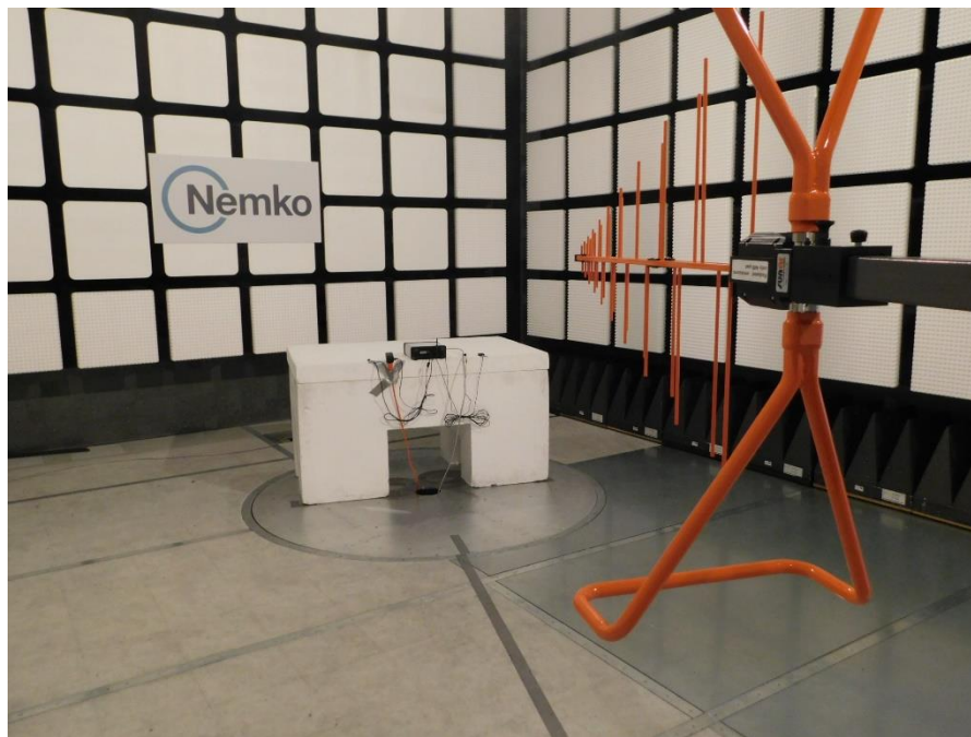
Figure 8.1-37: Radiated disturbance setup photo (SRX1200)
