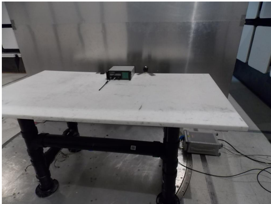
Figure 8.2-6: Conducted disturbance at mains port setup photo
