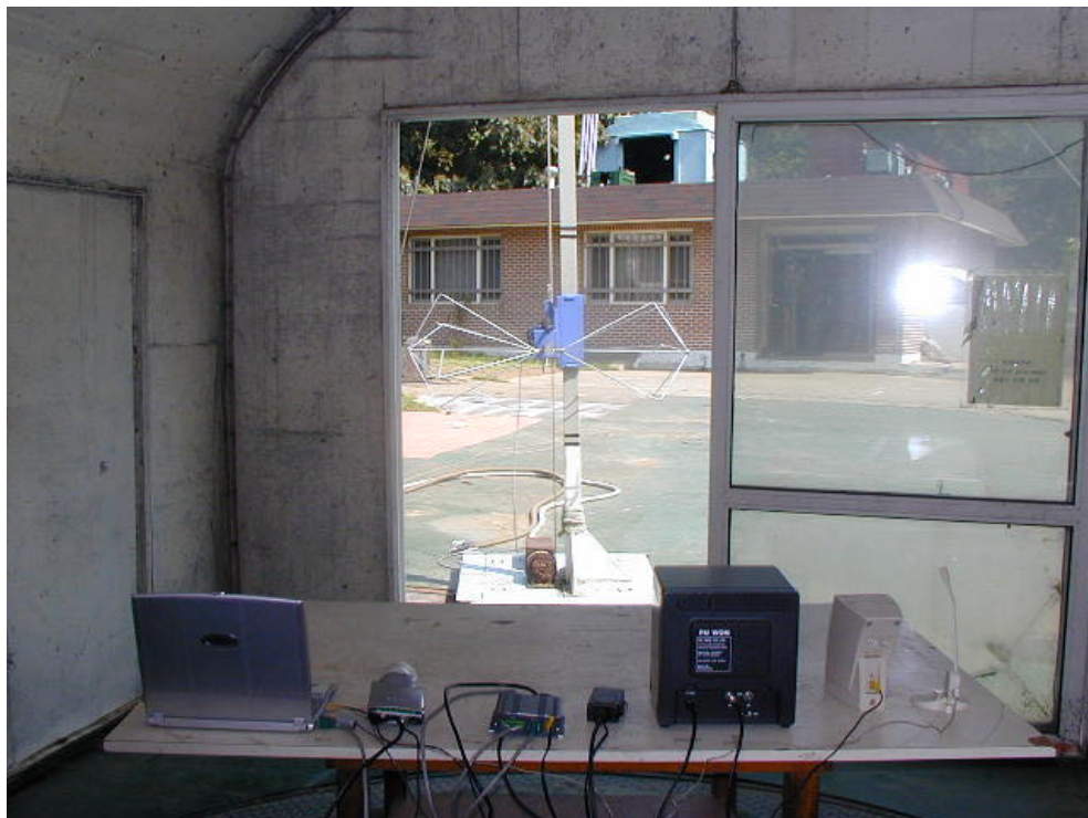
RADIATED EMISSION SETUP PHOTOGRAPH - REAR VIEW ( 30 - 300 MHz )
