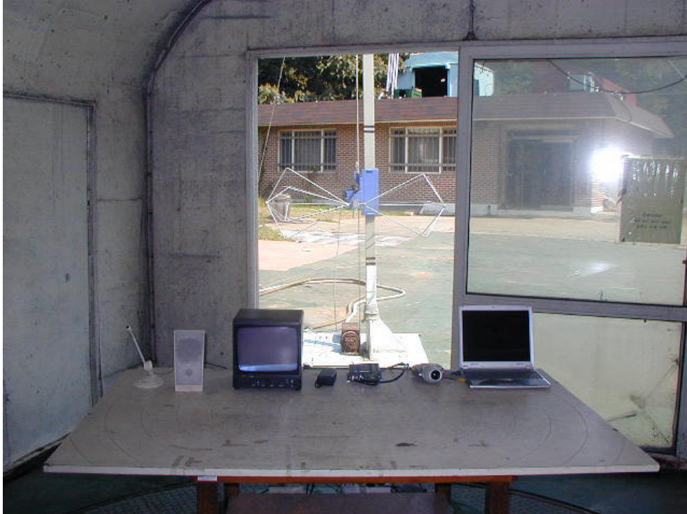
RADIATED EMISSION SETUP PHOTOGRAPH - FRONT VIEW ( 30 - 300 MHz )
