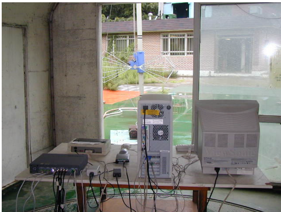
RADIATED EMISSION SETUP PHOTOGRAPH - REAR VIEW ( 30 - 300 MHz )
