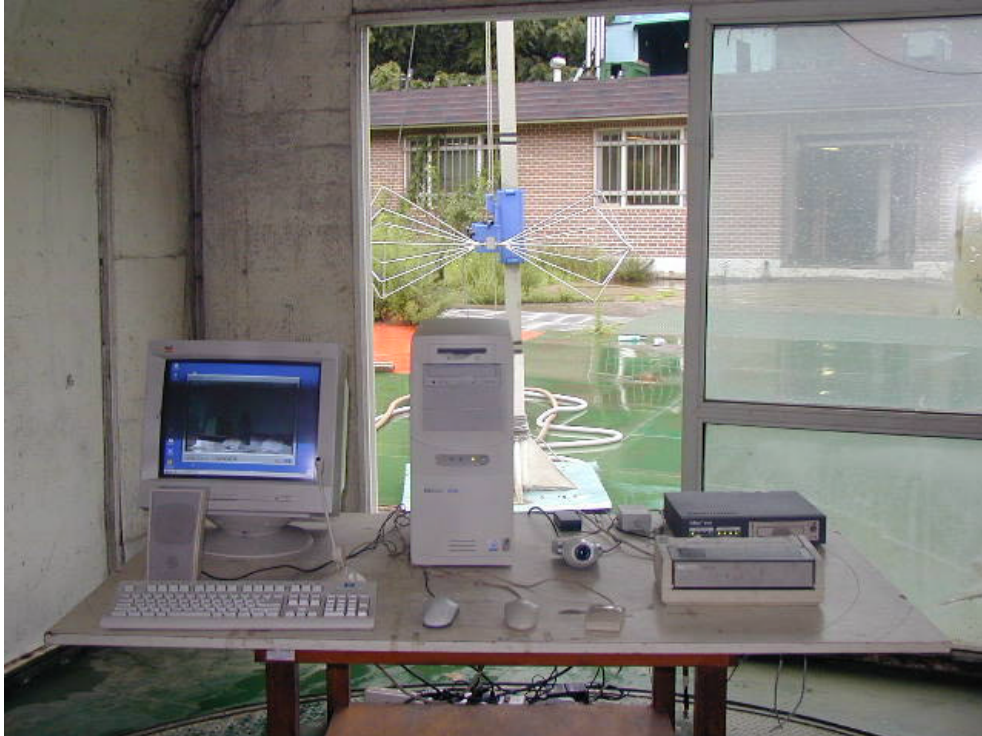
RADIATED EMISSION SETUP PHOTOGRAPH - FRONT VIEW ( 30 - 300 MHz )
