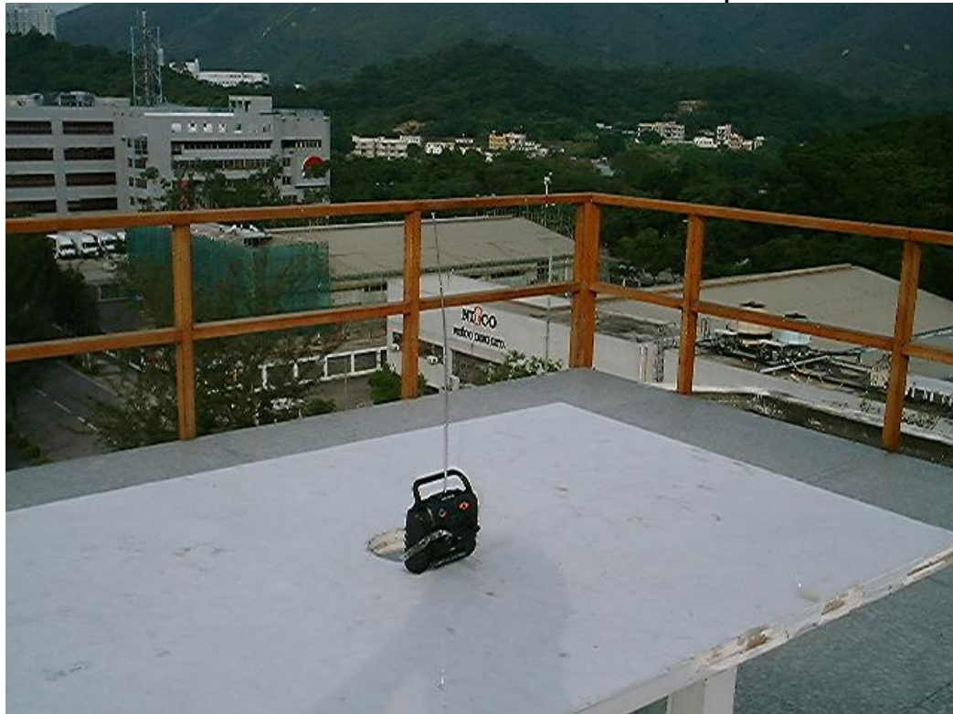
Measurement of Radiated Emission Test Set Up
