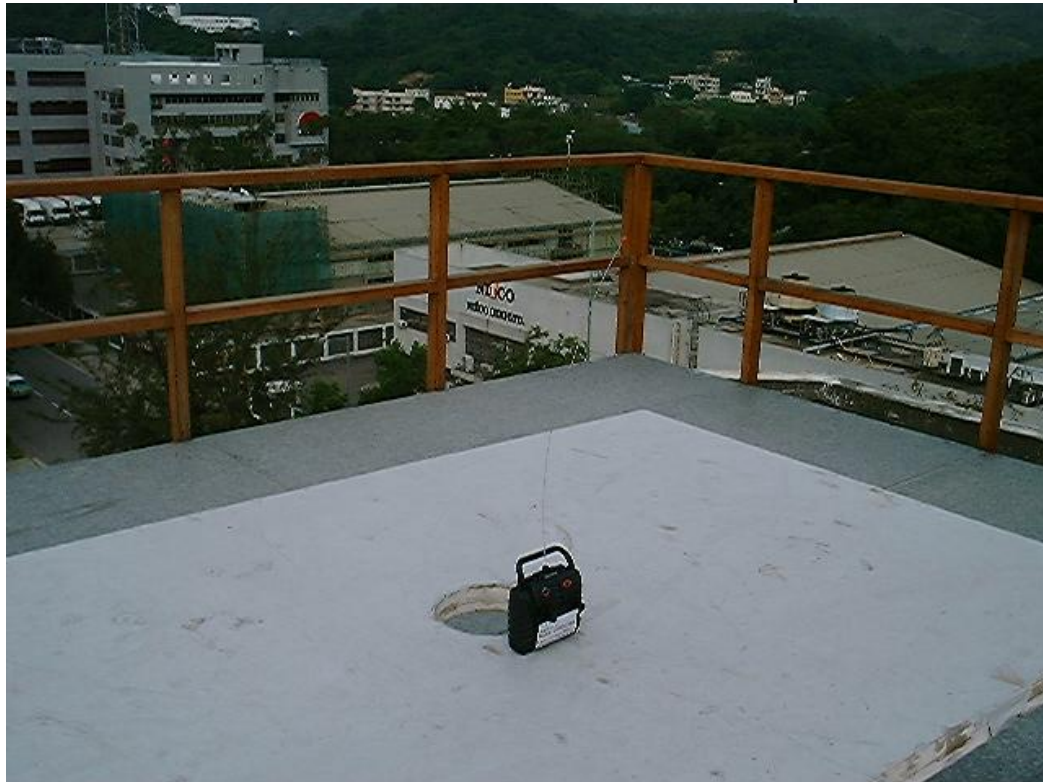
Measurement of Radiated Emission Test Set Up
