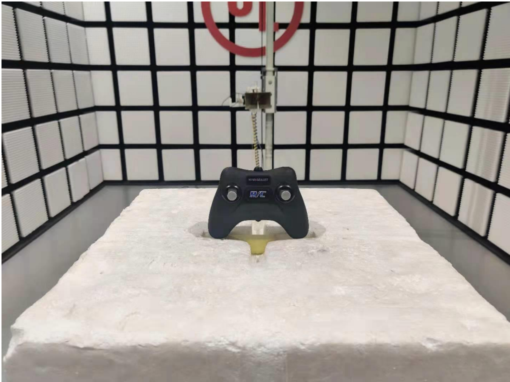
Radiated Disturbance Setup (Above 1 GHz – Y axis)
