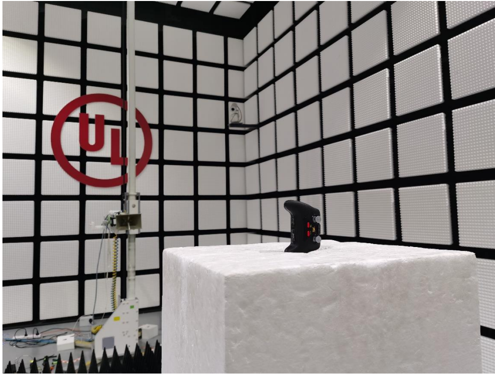
Radiated Disturbance Setup (Above 1 GHz – Z axis)
