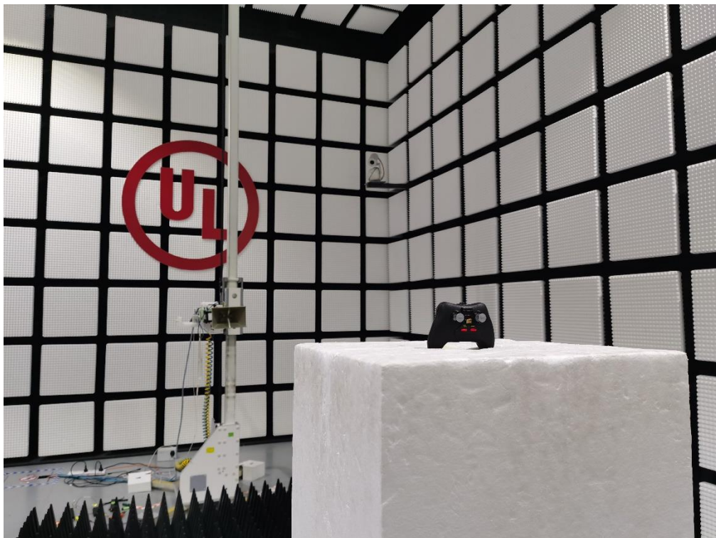
Radiated Disturbance Setup (Above 1 GHz – Y axis)
