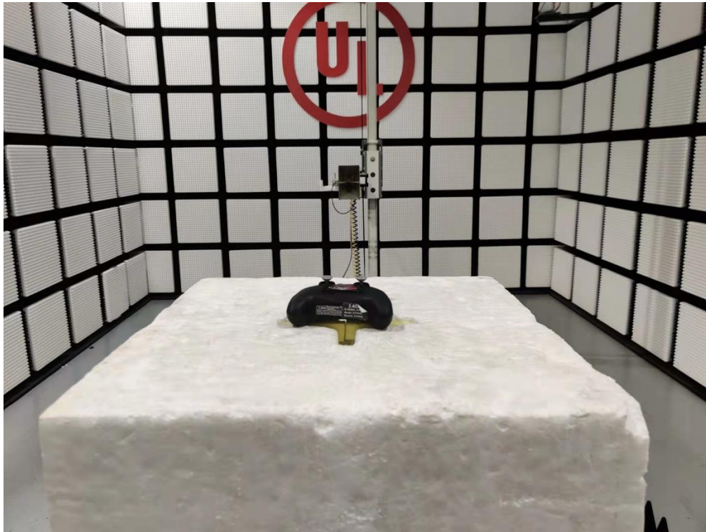
Radiated Disturbance Setup (Above 1 GHz – Y axis)
