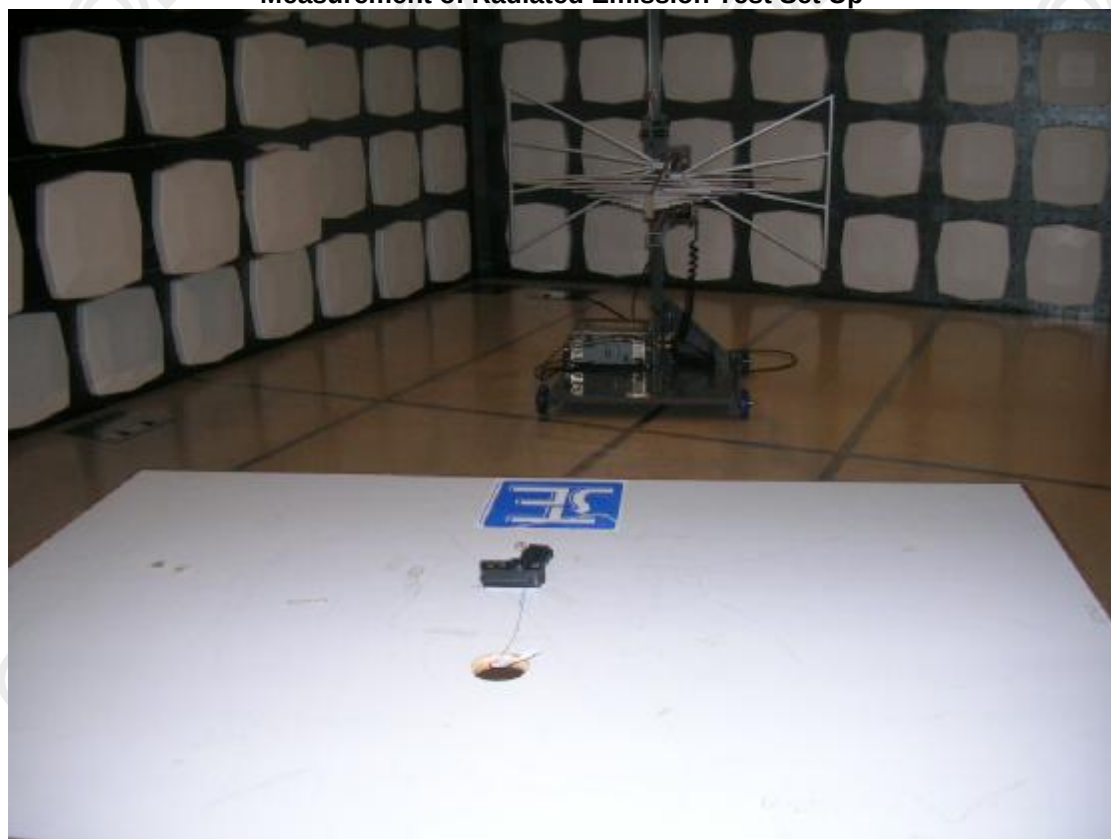
Measurement of Radiated Emission Test Set Up
