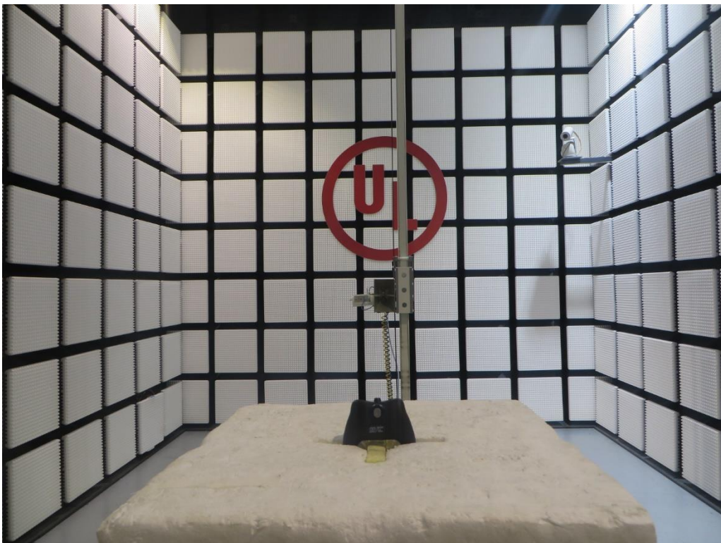
Radiated Disturbance Setup (Above 1 GHz-Y axis)
