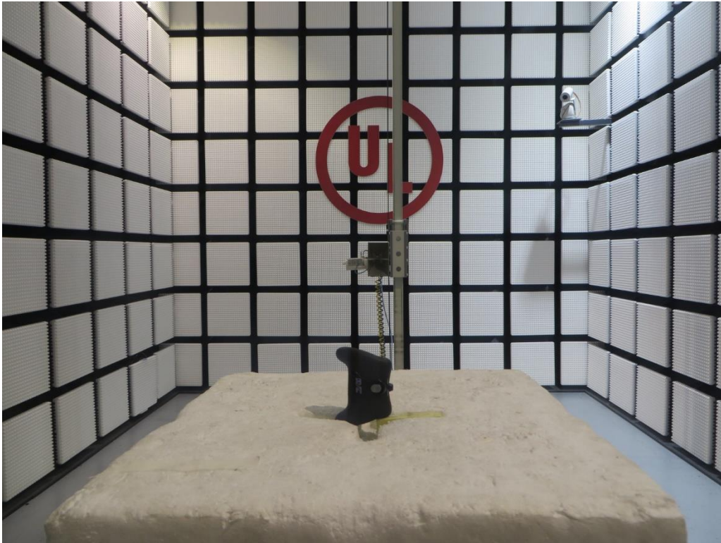
Radiated Disturbance Setup (Above 1 GHz-Z axis)
