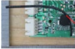
Wire Antenna: 60mm AWG22 PVC/Copper
