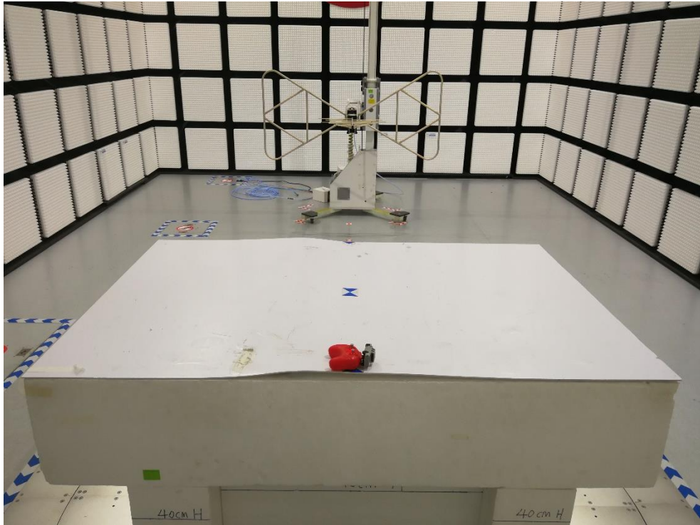
Radiated Emissions below 1GHz test setup photo
