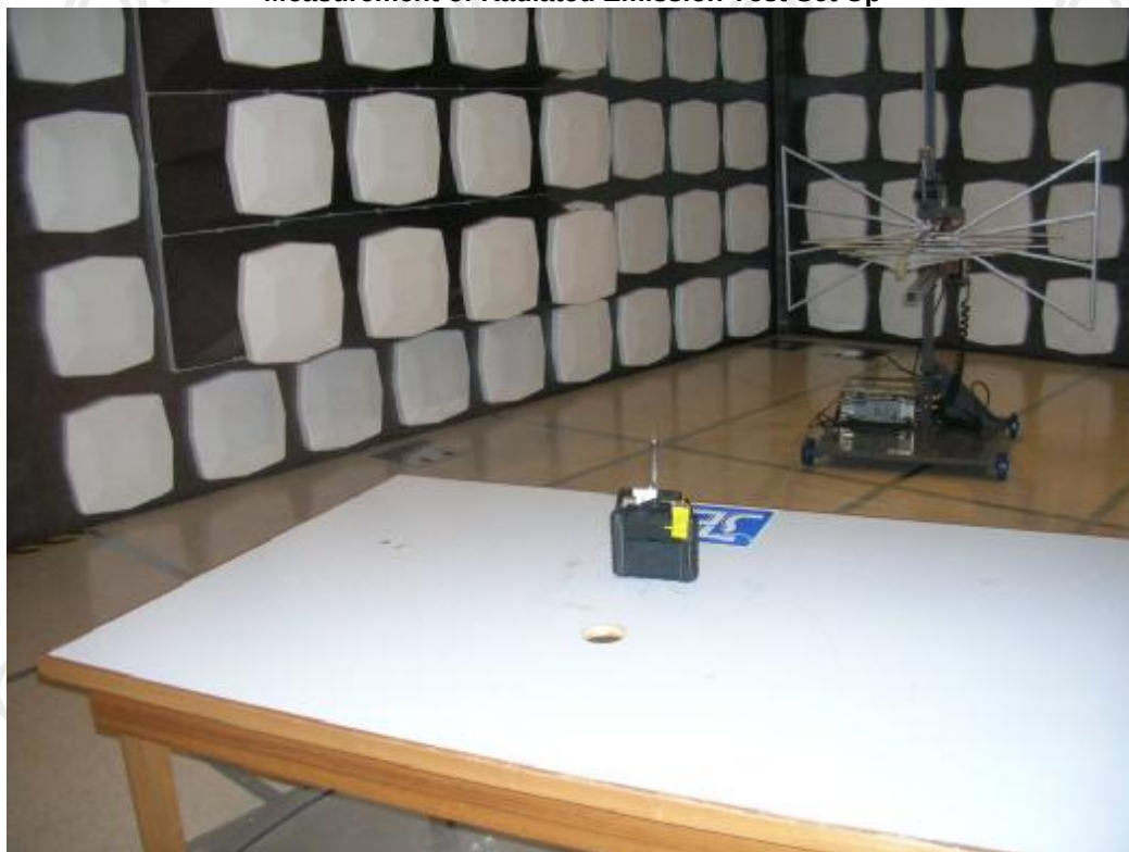
Measurement of Radiated Emission Test Set Up
