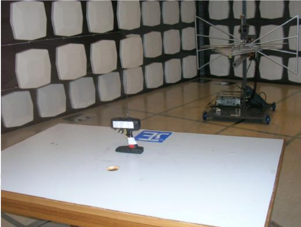
Measurement of Radiated Emission Test Set Up
