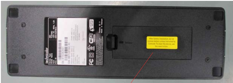
Battery label Position 貼于label框內
