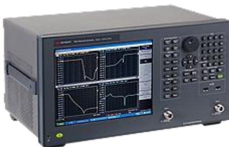
Figure 2 : Network analyzer used (Keysight E5063A).
