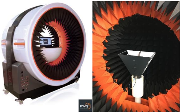
Figure 3 : Anechoic chamber used (MVG/Starlab).
