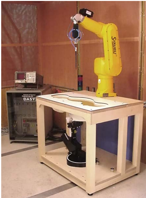
DASY3 SAR Measurement System with SAM Phantom
