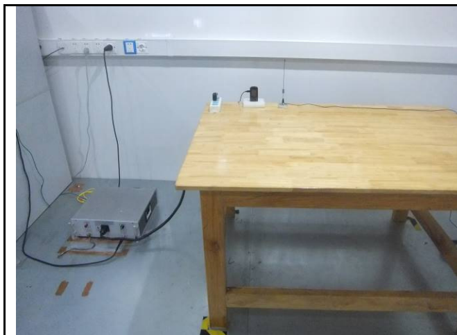
Conducted Emissions Test Setup Front View
