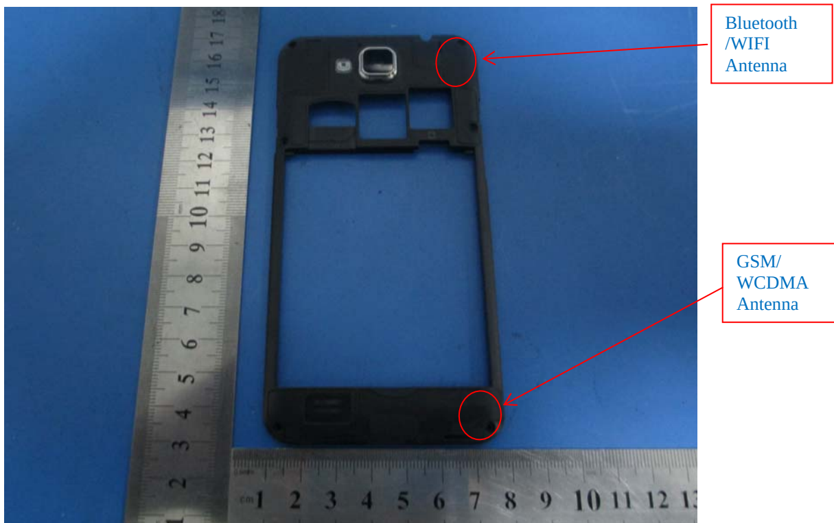
Antenna – Top View
