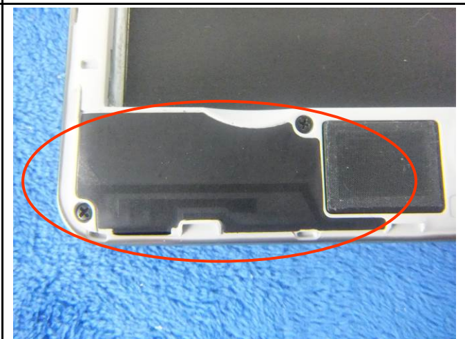
GSM/PCS/UMTS-FDD Antenna View
