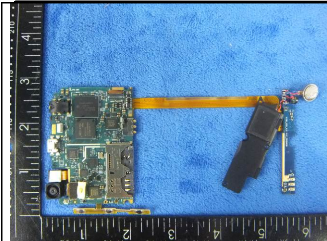
Mainboard Without Shielding - Front View
