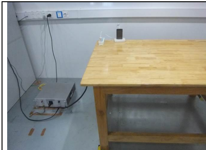
Conducted Emissions Test Setup Front View
