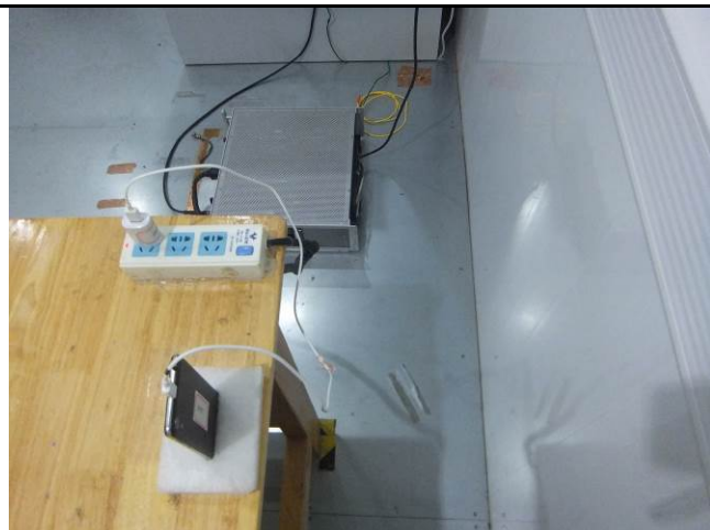
Conducted Emissions Test Setup Side View
