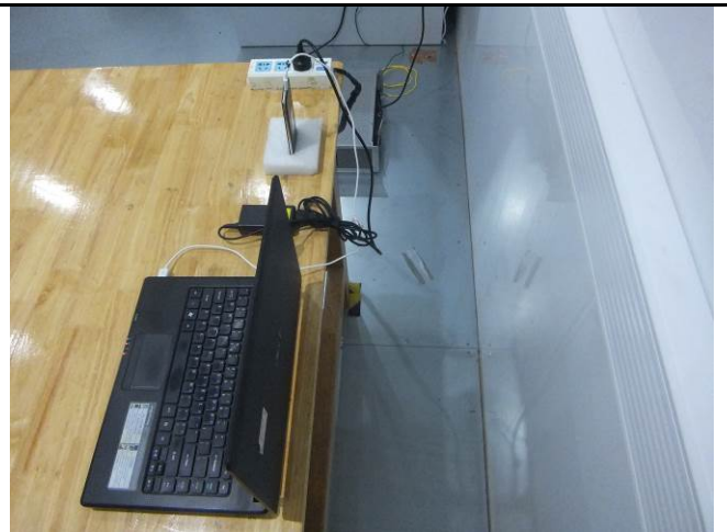
Conducted Emissions Test Setup – Side View
