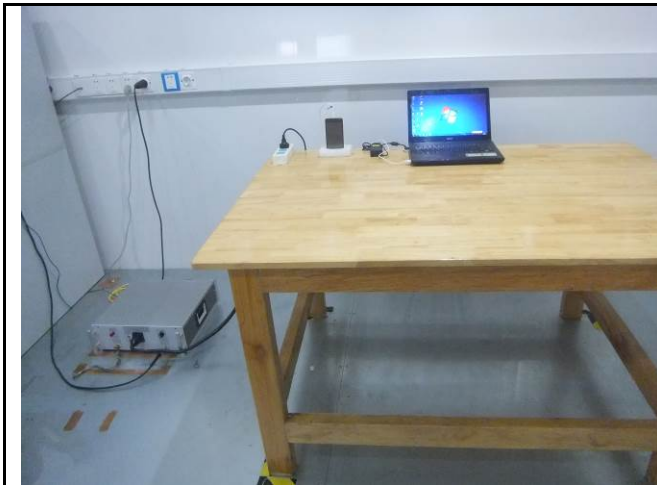
Conducted Emissions Test Setup – Front View
