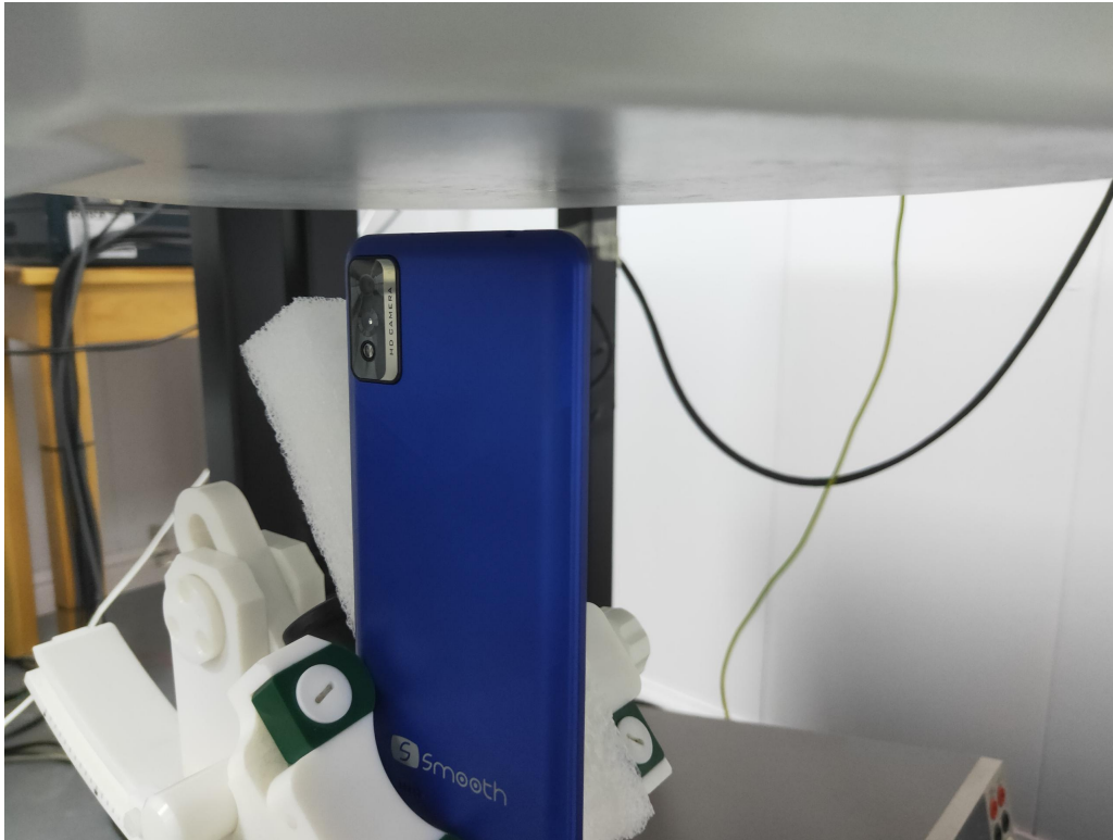
10mm body-worn Top Side Setup Photo (hotspot)
