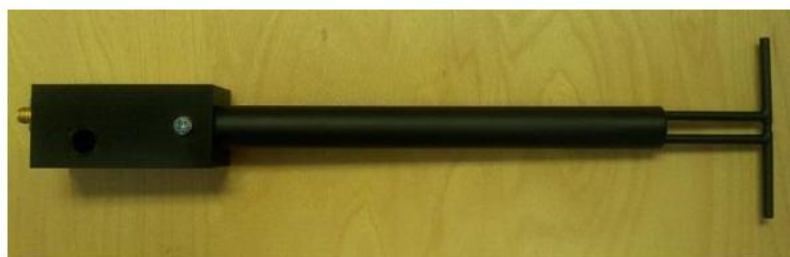
Figure 1 – MVG COMOSAR Validation Dipole
