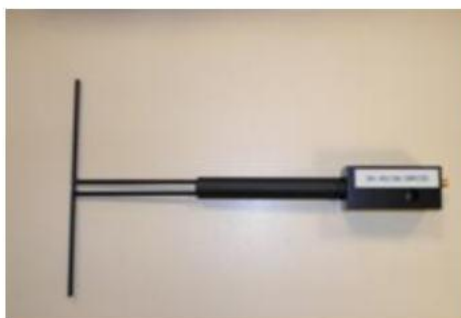
Figure 1 – Satimo COMOSAR Validation Dipole
